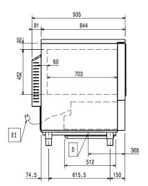
Drain Electrical inlet (power)
